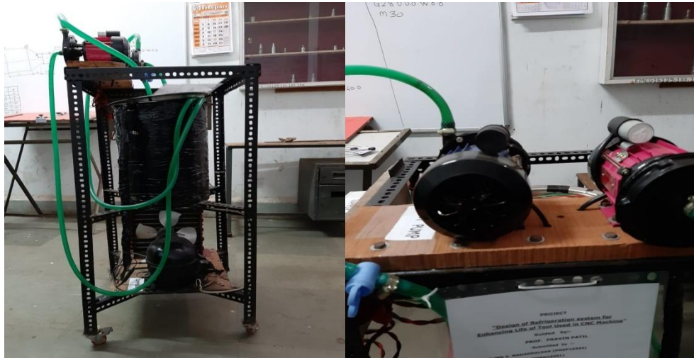
Figure 1. Refrigeration Coolant System along with Pressure Generation System
